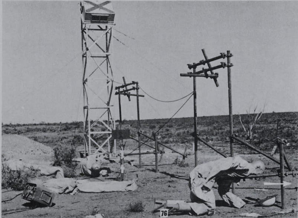
FIGURE 12. ROUND 2. DUMMIES AT 3100 ft AFTER FIRING. NOTE CROUCHING FACING DUMMY HAS REMAINED ON THE SUPPORT AND HELMET HAS DROPPED OFF AFTER POSITIVE PHASE
